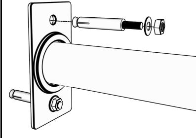
INSTALL CONCRETE SCREWS INTO PRE-DRILLED HOLES IN CONCRETE AND FASTEN NUTS UNTIL SECURE
