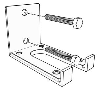
LOCATE WOOD STUD AND FASTEN WOOD SCREWS UNTIL SECURE
