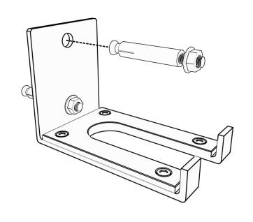
INSTALL CONCRETE SCREWS INTO PRE-DRILLED 1/2" HOLES IN CONCRETE AND FASTEN NUTS UNTIL SECURE
