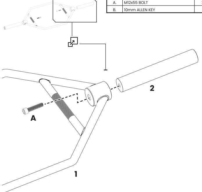
Insert the M12x55 bolt as shown into the sleeve and tighten with the provided Allen key. It is recommend to use a torque wrench to tighten to 40 ft/lb for safe assembly. Repeat on other side when completed.
