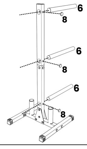
Align and center the plate loaders to the inside of the bar frame as illustrated.
