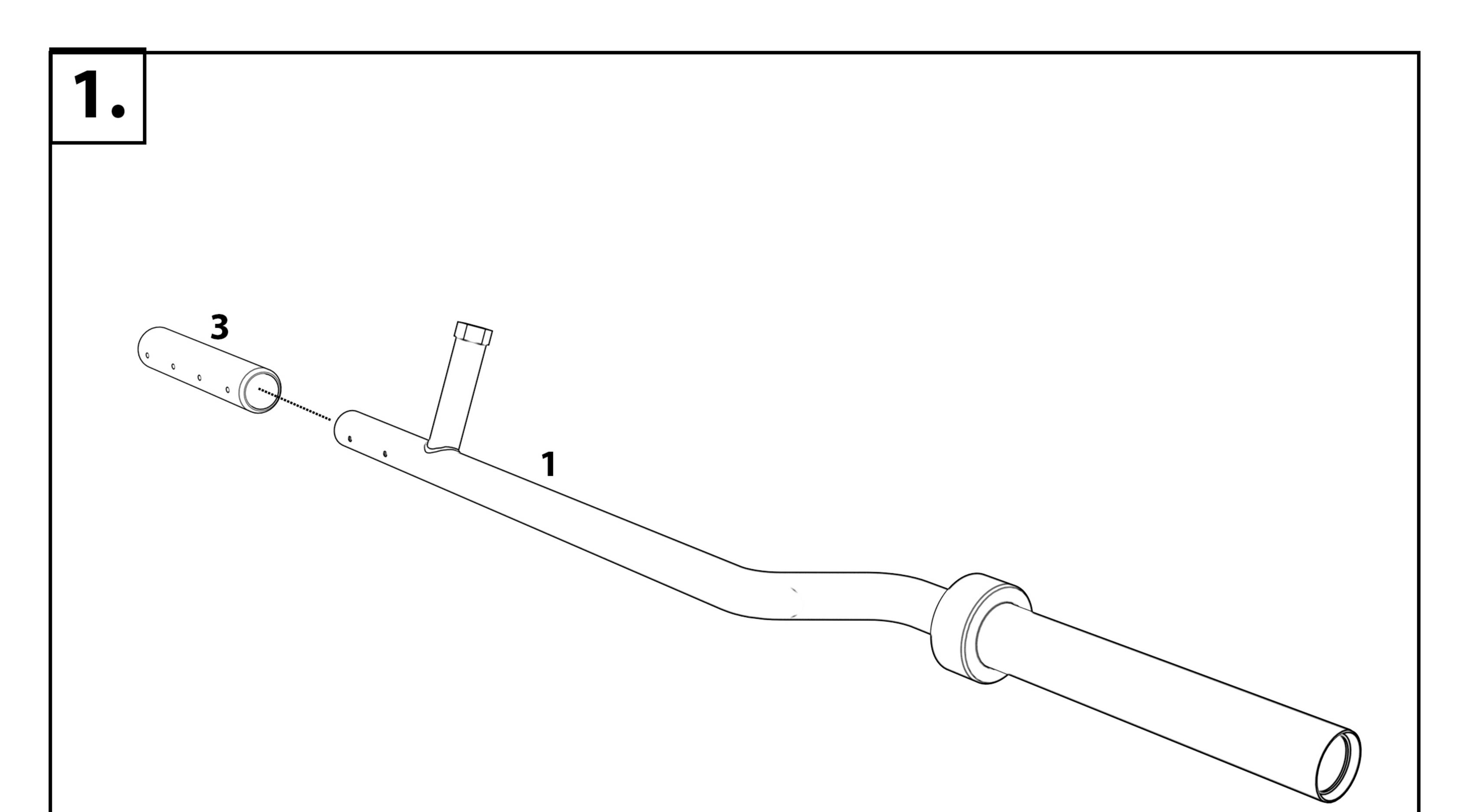
One at a time connect the bars to the connector piece (3).
